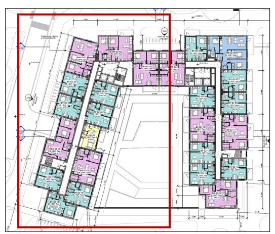
Figure 3.7: Extract from Block 05, Second Floor, GA Plan Dwg. No. DCD-RAU-02-B05\_02-DR-A-1502 showing 13 units per core.
